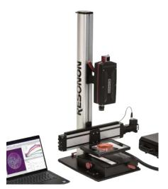
This system allows for illumination from above (Reflectance) or from below (Transmission). A clear sample plate is mounted to the linear stage, which is mounted on the column. The line light is easily transferred between the Reflectance and Transmission configurations.
