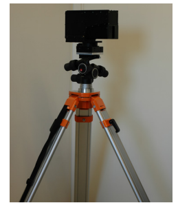
Figure 4. HySpex mounted on rotation stage and tripod.
